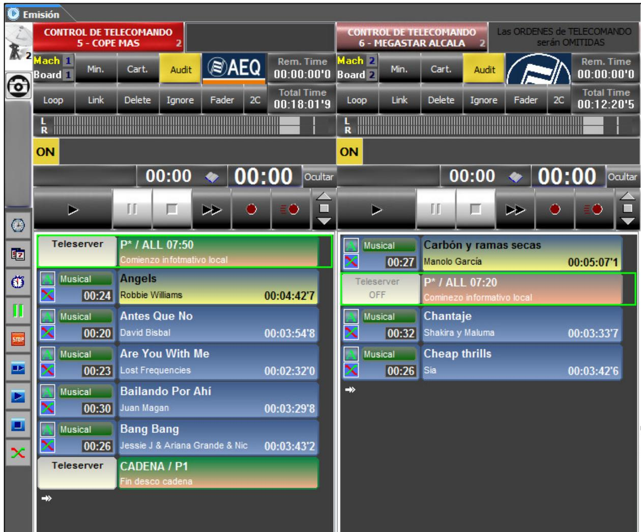
A new “REMOTE CONTROL COMMAND” button appears on top of any of the playout machines configured with Remote Control Commands, together with the description of the program it manages.
