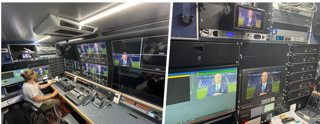
On-board system: Left photo, camera operator, video switcher and producer positions. Right photo: Crossnet intercom matrix.
