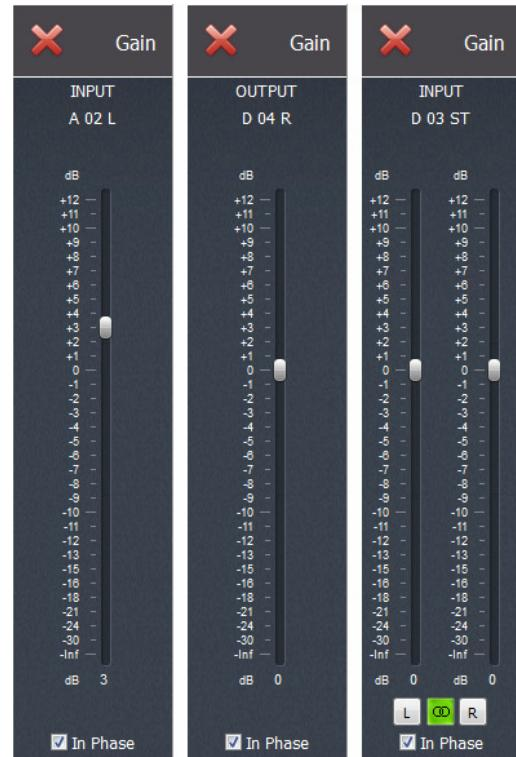
In the case of **stereo** lines the gain of each channel can be configured separately. In the lower part of this window 3 buttons are shown:
