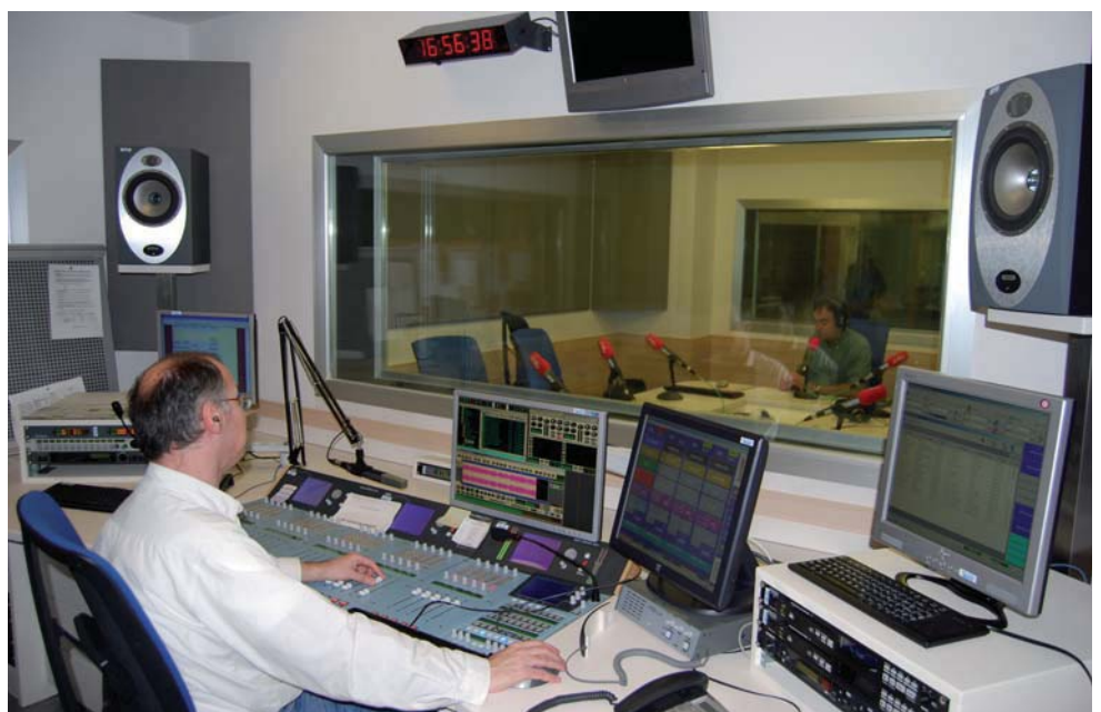
The main studio has two live broadcasting sets (for news and programs), four control-live broadcasting set studios, three studios for self-monitoring and four recording booths. Each of the booths is equipped with a "mini" AEQ Arena console with Eagle Real-time Control for recording telephone calls
