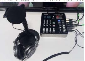
For control and mixing of the International Sound packages delivered by OBS in MADI format with the Spanish Language Commentary audio, Claro Sports used an AEQ ARENA digital console with 15 motorized faders and capability of up to 9 pages. A multi-
