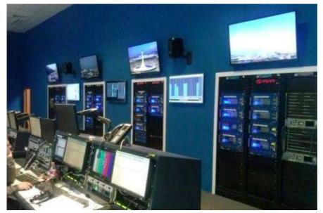
Of the more than 80 international broadcasters deployed in Sochi, about 55 were equipped with an AEQ digital audio panel (DAP) at their facilities in IBC or MBC. The DAP consist in of a chassis BC2000D router and fitted with audio input and output cards to comply requested with the services and audio channels provided by the Host Broadcaster. including those from the
