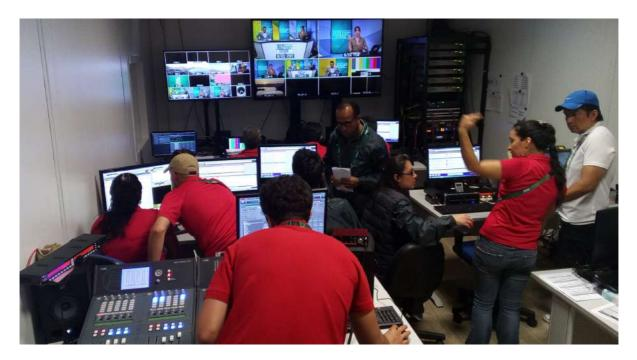
Quality control was accomplished with an AEQ CAPITOL IP mixing console connected to the AoIP Network in combination with DANTE<sup>TM</sup> Virtual soundcard application installed on computers for the discreet monitoring of any signal available on the AoIP multi-channel network.
