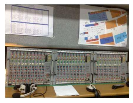
For venues interconnectivity and international contribution AEQ also supplied 35 PHOENIX STUDIO, a multi-format, multi-algorithm dual channel audio-codec designed for stationary rack-mounted applications, like links between studios or STL. PHOENIX STUDIO offers the options of working over ISDN and IP networks, among many others. The IP communications interface is fully compatible with the EBU-TECH 3326 technical specification issued by the EBU N/ACIP working group.
