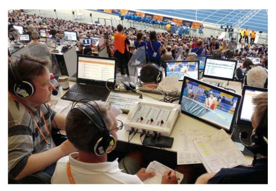
The entire AEQ OLYMPIA 3 system works over IP networks using DANTE – AES 67 protocol for the transmission of multichannel audio, what makes dynamic signal routing much easier. The system was supported totally by remote control from one or several distributed PCs.
