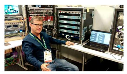
Each AEQ Phoenix VENUS is capable of establishing 4 simultaneous bi-directional mono channels to two different destinations so the 16 channels of commentary audio fitted snugly into the 4 Units at each end.
