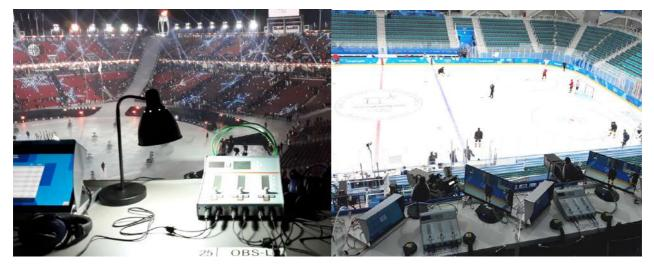
The magnitude of a system like this is difficult to comprehend. In excess of 100 BC2000D chassis with 268 redundant fiber MADI interconnection links and high-speed links with capacity of 1024 Audio channels were deployed to inter-connect audio distributors and concentrators.
