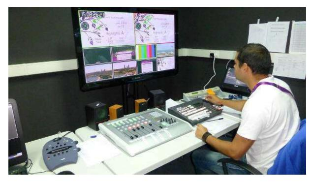
The supply was completed with an AEQ DCS-10 Commentary System used for all "off-tube" booths at IBC. The system also rendered commentator service for the host organization for the news channels and direct feeds available during events for, for example, ASBU - Arab Broadcasting Union and English speaking Broadcasters.
