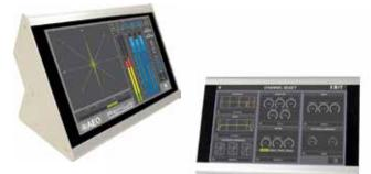
The ATRIUM console incorporates the specific features for ON AIR broadcasting: automatic monitor mute, cough mute, fader start, control signalling etc. In addition, it incorporates programmable keys to control external equipment: communications, intercom, visual radio. At the process level, it has an immense capacity for adjusting frequency, dynamics, multi-band mixed process, delay and reverb. Also unattended mixing is enabled through autogain and automix functions.
