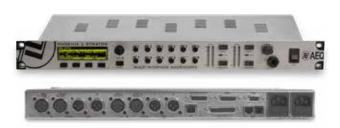
Additional connection for ISDN and X21/V35 lines and physical user interface on the front panel.
