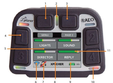
1 Programmable key. 2 Status indicator. 3 Programmable key. 4 4 programmable shortcut keys, or channel selection in Party-Line mode. 5 2.4" TFT screen. 6 Wi-Fi signal level indicator. 7 Mute indicator. 8 Terminal name tag. 9 Battery level indicator. 10 4 LED mode indicators. 11 Input level indicator for each interlocutor.
